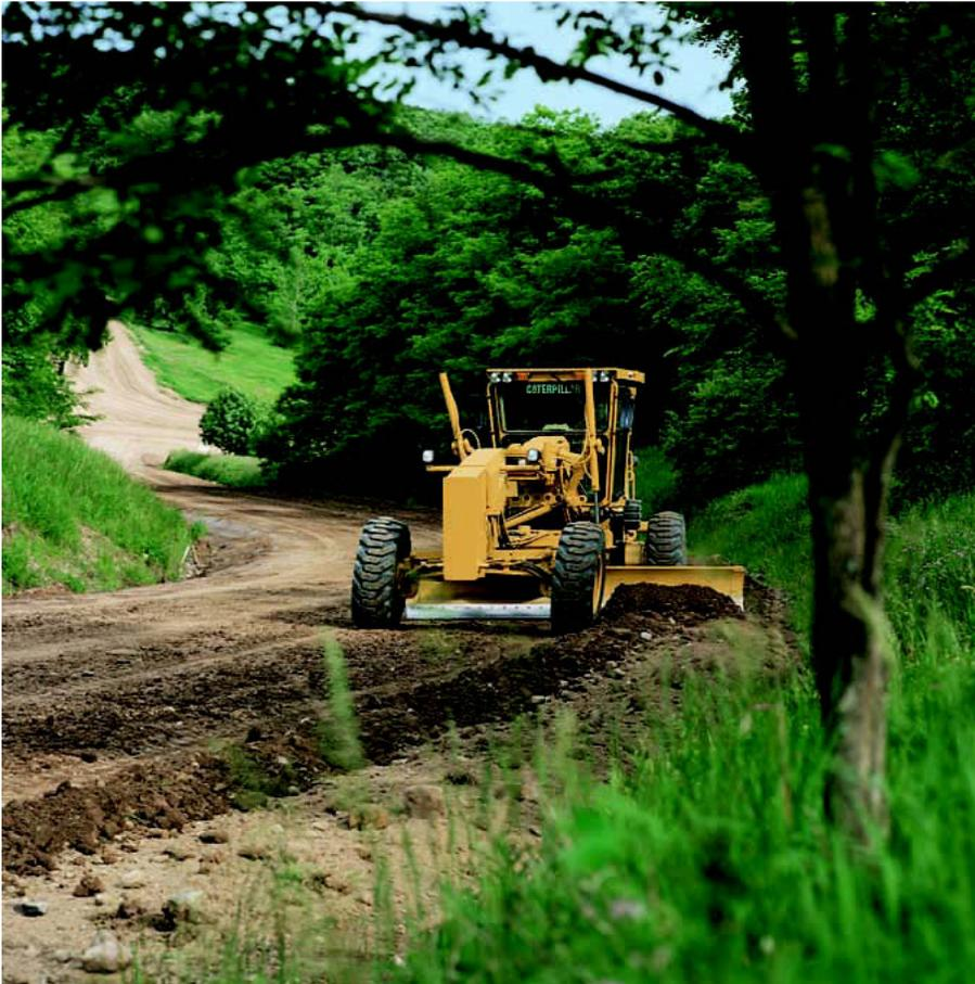
**Quiet Cab.** The resiliently mounted engine and transmission reduce interior engine noise and vibration to less than 75 dB(A). With the sound suppression group, interior sound levels do not exceed 72 dB(A), using ISO 6394. Lower interior noise levels improve operator working conditions.
