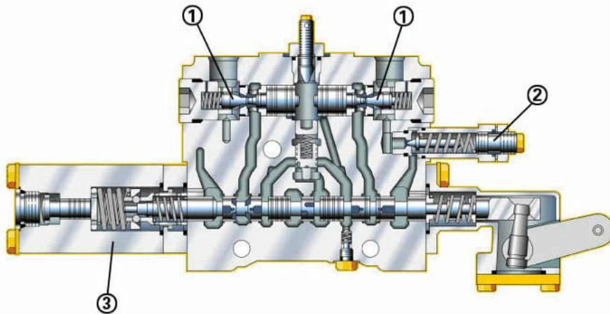
1 Lock valve, 2 Line relief valve, 3 Blade float detent
